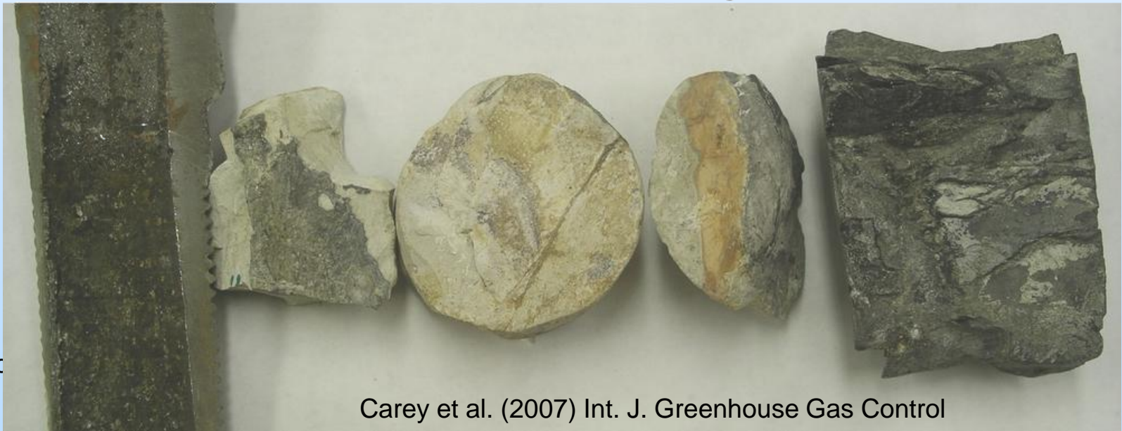
Casing Cement with Rind Cement with Vein Cement Orange Zone Shale Fragment Zone Shale Fragment Zone and Shale
